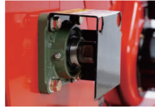
Imported high speed bearings High concentricity, tight collection, wear-resistant and durable
